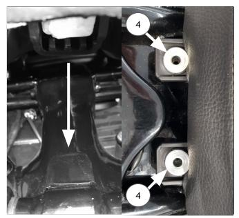
**6** Insert the 2x Hex Flange Head Bolts (3) that were removed earlier and torque to **12NM**
