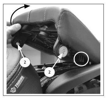
**3** Remove the 2x Hex Flange Head Bolt (3) and 2x Sleeve (4) from the rear of the rider's seat and retain for refitting the seat
