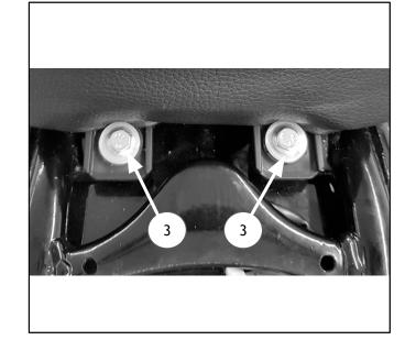
**7** Refit 2x top hat inserts (2) into grommets in the passenger Seat.
