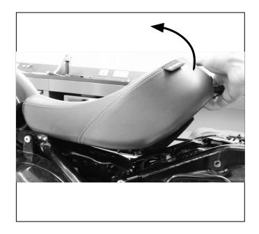
**5** Push the front of the new accessory rider's seat on to the fuel tank tab and align rear mount point to the frame. Refit 2x top hat inserts (4)
