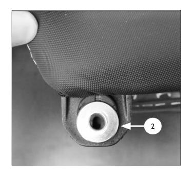
**8** Re-insert the rear passenger seat hook into the frame and align the front mounting holes.
