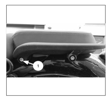
**2** Lift the front of the passenger seat and unhook from the frame. Remove top hat inserts (2) from left and right hand side. Retain for future use.
