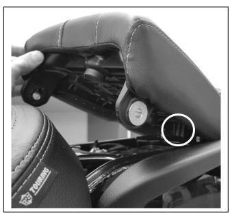
**9** Reattach passenger seat by reusing the CAP head Bolt (1) removed earlier. Insert through the grab rail boss and into the frame. Torque these to **25NM** and repeat on the other side.
