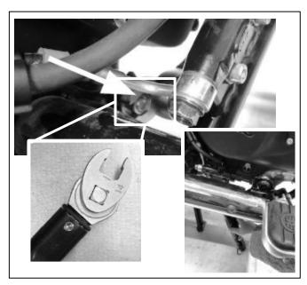
**3** Remove the front engine mount bolt (arrowed), Washer (3) and U nut (1). Assemble the front mount bracket (2) as shown, leaving the bolt loose at this stage.
