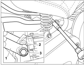
**7** Tighten the rear suspension fixings (1) on both sides of the motorcycle to **40 Nm**, right hand side shown.
