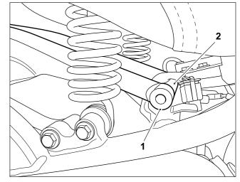
**5** Lower the luggage rack (1) and slide the rack forwards to engage the mounting brackets (2) on the rear suspension fixings (3), right hand side shown. Ensure the mounting brackets are located behind the washers (4) on the rear suspension fixings, as shown.
