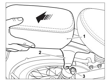
**4** Carefully position the luggage rack front mounting bracket (1) under the rider seat and locate the mounting bracket correctly on the frame mounting (2).
