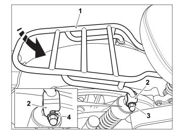
**6** Align the front fixing positions of the luggage rack (1) with the mounting position on the motorcycle frame (2).
