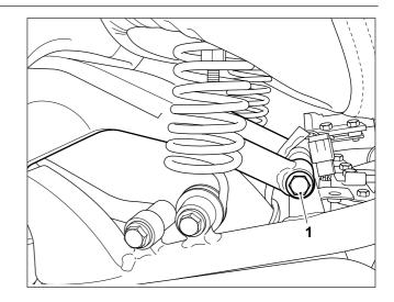
**2** Loosen the top rear suspension mounting nuts (1) on both sides of the motorcycle, right hand side shown.
