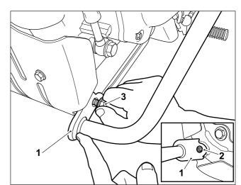
**4** Align the bottom mounting of the engine guard (1) with the mounting point on the motorcycle frame (2), as shown. Fit an M8 x 12mm fixing (3) from the kit. Tighten the fixing to **16Nm**.
