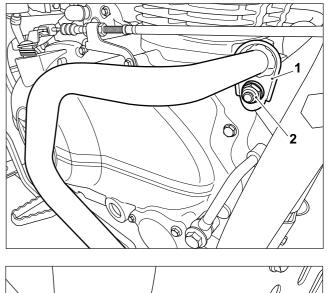
**6** Align the bottom mounting of the engine bar (1) with the with the mounting point on the motorcycle frame (2). Fit an M8 x 12mm fixing (3) from the kit.
